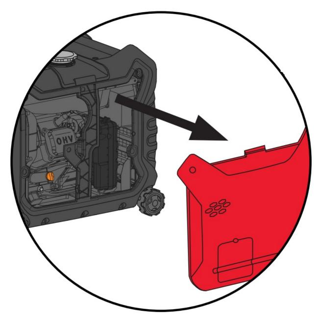
2. Pull the Oil Drain Hose out of the Generator. Remove the Oil Drain Cap. Drain Oil. Replace the Oil Drain Cap. Put the Oil Drain Hose back into the Generator and fill oil.
